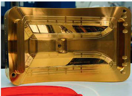
A mould coated with TiN-ultrafine for use in plastic injection (in front the fabricated plastic cover for the automobile sector).
